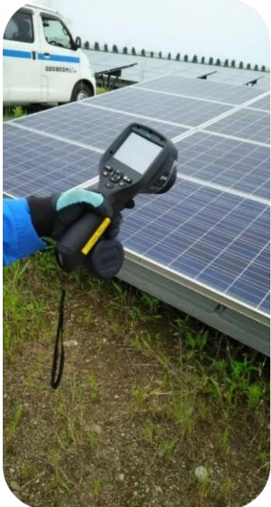
Inspection performed using thermal imaging camera
